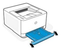
b. Press and hold the button on one of the paper-width guides and slide the guides to the edges of the input tray. Do the same for the paper-length guide.
