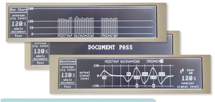
Other screens include: main menu, test signal level, spacing errors, bar chart, extraneous ink characters, field analysis and actual signal level.
